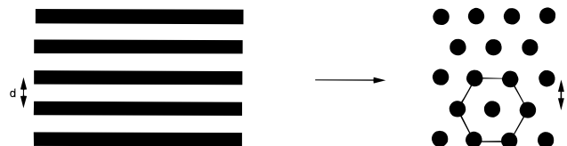
Figure 12. Epitaxial growth of a hexagonal-packed cylinder melt structure from a lamellar solid structure. The X-rays are incident in the direction of the arrow.
